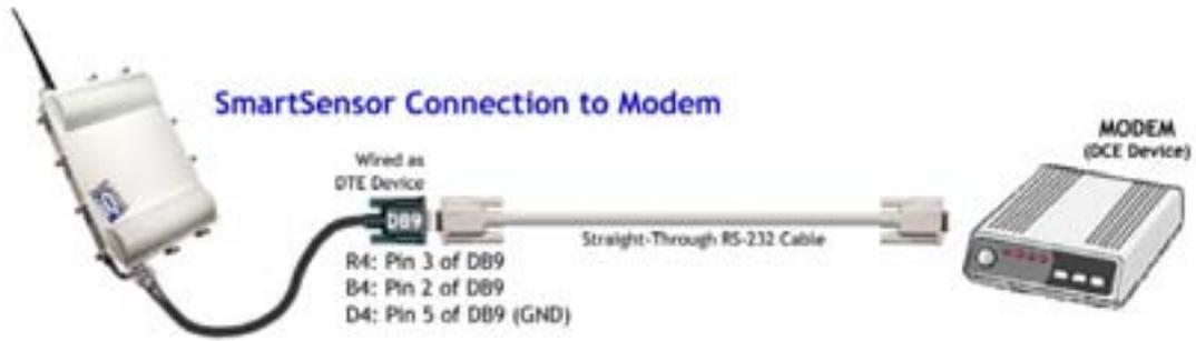
Figure 35 - Connecting a Modem to the SmartSensor
